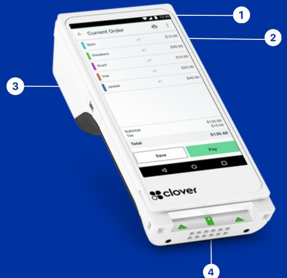
1. Built-in Camera & Barcode Scanner
